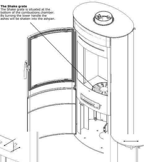
The Shake grate Operate by moving the handle inn and out.
