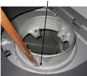
Make an opening using chisel or similar.
