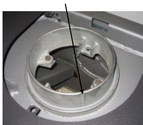
Marking of condensation drain.
