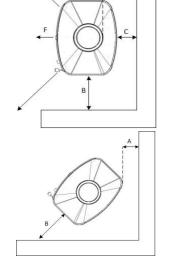
The stove must in accordance with applicable rules comply with the following minimum distances from inflammable walls and materials:
